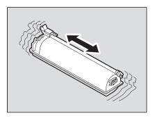
**5** Pull out the seal in the direction of the arrow.
